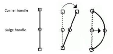
You can also modify primitive shapes by typing in new coordinates and bulge values in the value bar.
